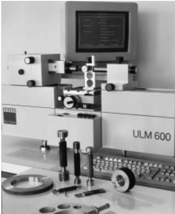
Zeiss Universal Length Measuring Machine ULM 03-600
