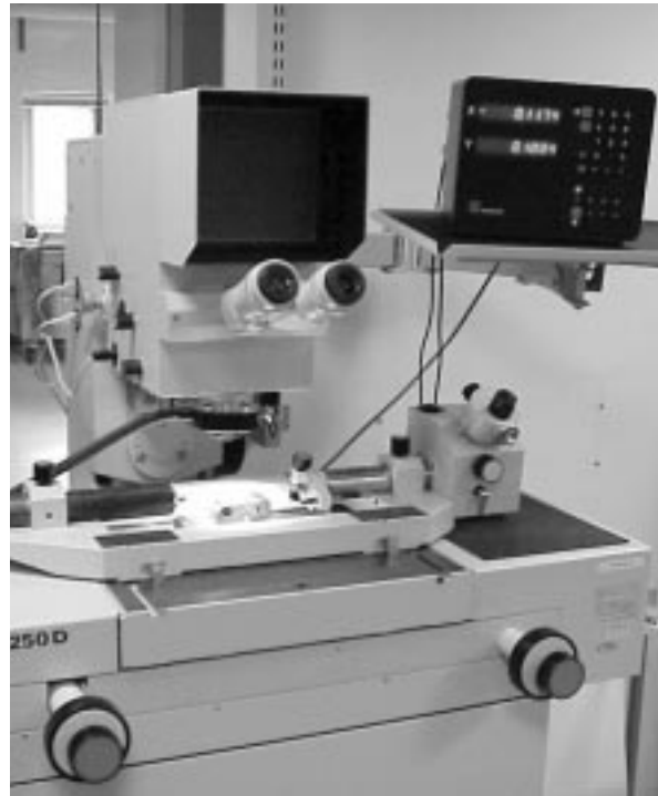
Zeiss 2 co-ordinate Measuring Machine ZKM 01-250
